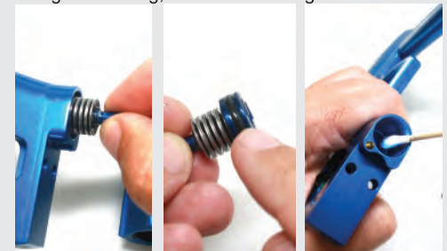
3. Remove reg piston. Clean and grease o ring, stem and housing.
