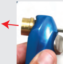
4. Remove brass adjuster housing by pressing it out of the ASA using a 1/8 allen wrench.
