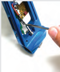
2. Remove ASA screws using 1/8 allen wrench
