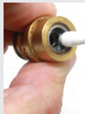
5. Clean and grease the o-ring inside the adjuster housing using a swab. Clean the reg seat at the bottom of the adjuster housing assembly.
