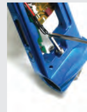
7. Press reg assembly and ASA back into the bottom of the grip frame and firmly tighten the mounting screws.
