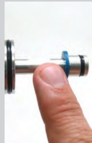
5. Apply light grease to Ram Shaft
