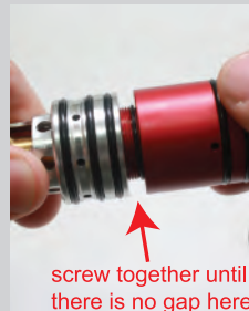
8. Tighten engine halves together until very tight
