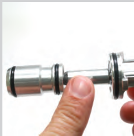
7. Apply light grease to Bolt Stem and o-rings
