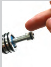
4. Apply light grease to ram U-Cup
