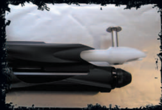
Lift Bolt Pin & Remove Bolt
