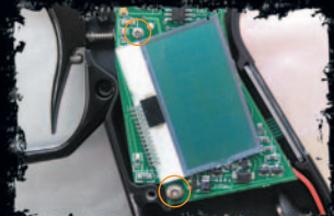
Remove Board Retaining Screws
