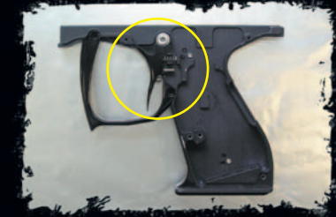
Remove Trigger & Spring
