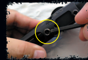
Remove Ram Sleeve Retaining Allen
