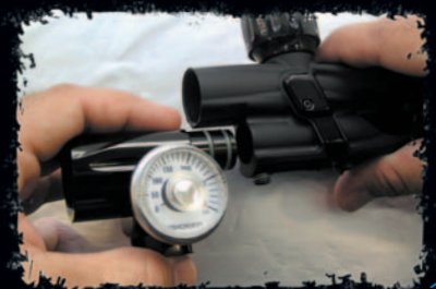
Remove ASA Block From Body
