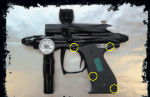
Separate Trigger Halves
