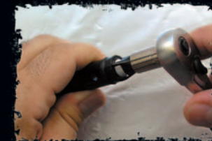
Loosen Valve Using 3/8" Socket
