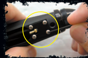
Remove Rear Air Barb Block
