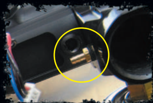
Remove Air Barb From ASA Block
