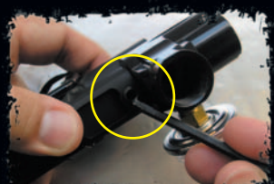
Remove LPR Retaining Allen
