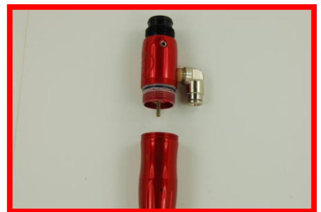
Disassemble the regulator by unscrewing the top and bottom halves then removing the internals. Tapping the bottom half into your hand will help the washer stack slide out
