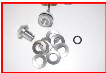
The shim stack disassembled. The retainer o-ring is the only one in the marker that does not get lubed.
