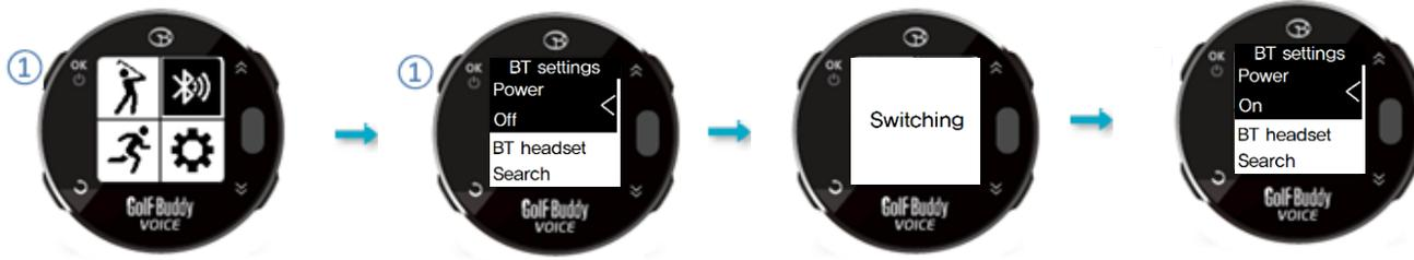
Press ① to enter BT settings. Press ① to switch the Power.
