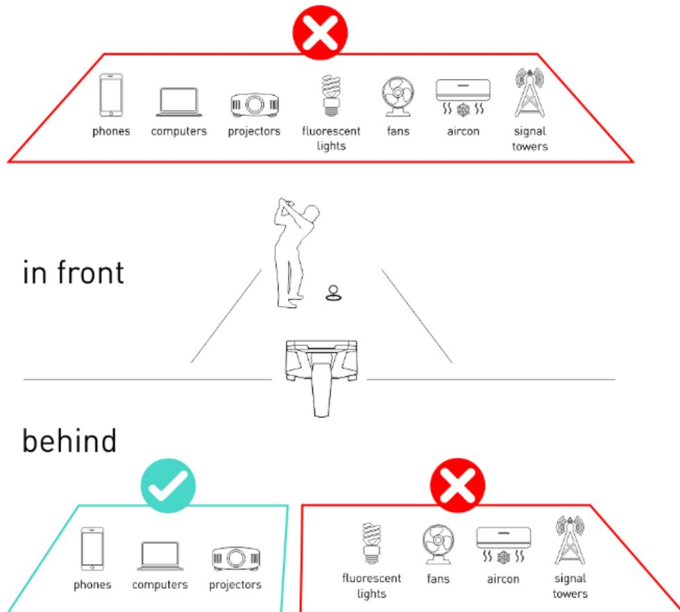
Try to prevent false triggers by switching such lights or machines off, or install a wire mesh screen in the light covers or over the interfering machines.
