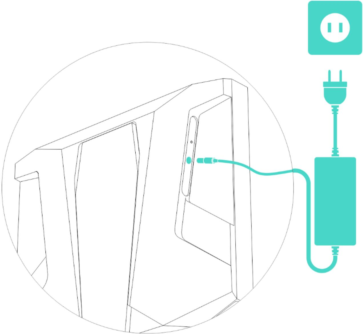
Charging the X3 to full capacity takes up to 10 hours using the supplied power adapter.
