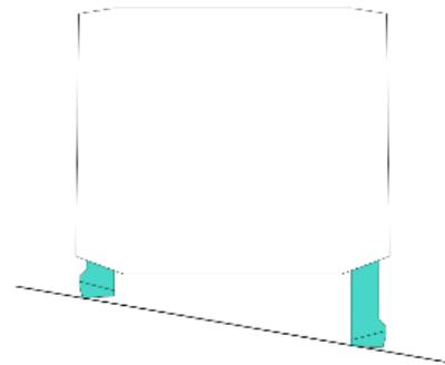
While starting up, the unit will automatically adjust its level according to the slope of the ground or floor.
