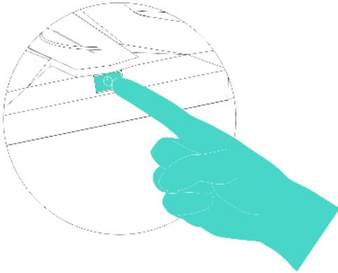
Hold the X3 unit, and press the latch under the unit to release the leg.
