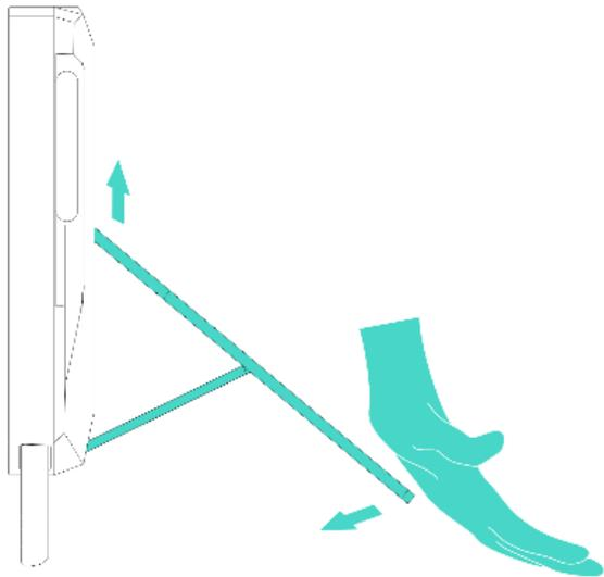
Lift the X3 unit and push the leg back to its closed position, until the latch clicks.
