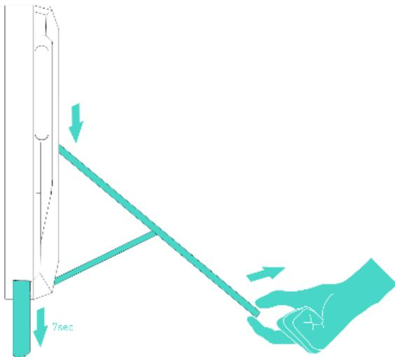
Pull the leg down and outwards until fully extended.
