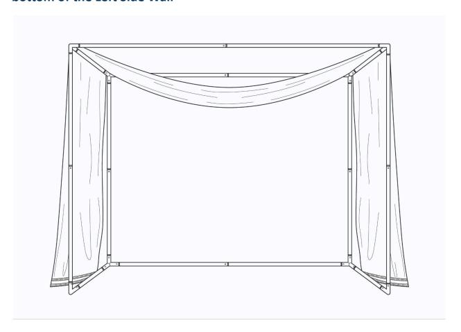
Step 5b: Disconnect the velcro on the end of the blackout curtain and pull underneath the left side wall (A-Frame Piece) and Reconnect the Velcro by Wrapping the End of the Blackout Curtain Around the Bottom of the Left Side Wall and Reconnect Velcro Securely
