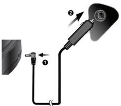
**Note:** Cord fits tightly into detector. When installing the cord, expect some resistance.
