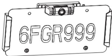
10. If needed, 2 cushions are provided to protect your vehicle. Attach to the back of the spacers containing the machine nuts.
