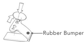
**IMPORTANT:** Some newer cars have a plastic safety coating on the inside of the windshield. The windshield bracket may leave permanent marks on this type of surface. To find out if your vehicle has this type of windshield, check the owner's manual or ask your dealer. We recommend that you do not leave the suction cup bracket on the window in direct sunlight. If the detector is removed, this may cause blistering of the dash in some vehicles.
