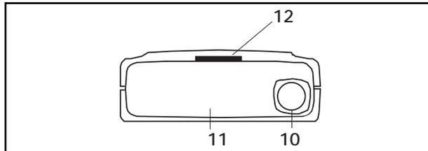
**10. Laser Antenna (Front)** – High gain optical lens array provides increased sensitivity and field of view for leading-edge laser detection.
