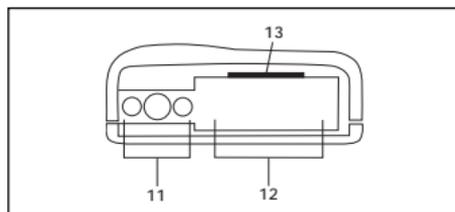
**11. Laser Antenna (Front)** - High gain optical lens array provides increased sensitivity and field of view for leading-edge laser detection.
