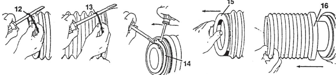
Slide the adaptor ring (15) off the spindle and remove it from the boot. Take the boot off the spindle (16).
