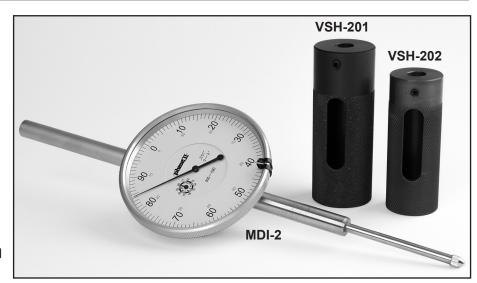
The **VSH-201** tube should have the dial indicator set for maximum reading (10 revolutions on gauge), then tighten dial indicator. This will set gauge to read from one inch to two inches.
