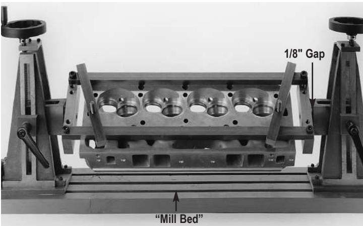
is required to lock the head securely in place.
