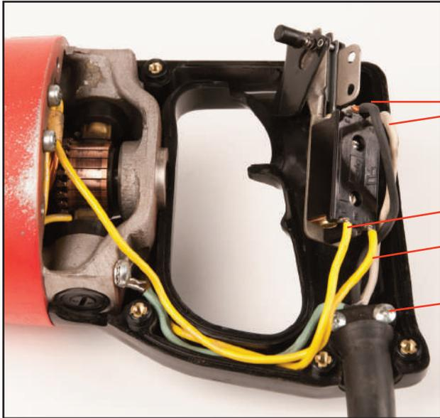
3. Remove these leads from switch. Refer to image at left and Illust. A.
