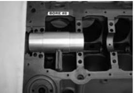
Fig #14 To clear for #8 rod keep the flange farthest from the pointer against main saddle #5.
