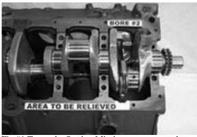
Fig #1 To set the Stroker Mimic we recommend creating a relief in the block for rod #2 at the pan rail area, using your normal process (crank, rod, piston and bearings).
