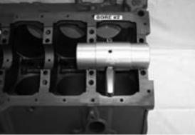
Fig #8 To clear for #2 rod keep the flange closest to the pointer against main saddle #2.
