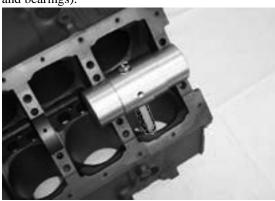
Fig #4 Rotate the arbor and adjust the pointer in or out until the tapered end of the pointer passes freely thru the relief with a minimum of clearance.
