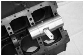
Fig #3 Place the arbor in main saddles #1 and #2 keeping the flange nearest to the pointer against main saddle #2.
