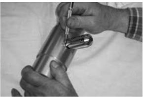
Fig #6 Once satisfied with the setting, scribe a line on the pointer opposite the set screw, utilizing the flat provided in the arbor or measure and record so it is possible to return to that setting for future use. Scribe or measure a different position for each new rod and stroke combination.
