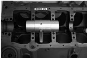
Fig #12 To clear for #6 rod keep the flange closest to the pointer against main saddle #4.
