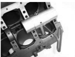
Fig #5 Lock the pointer in position with the set screw and check the clearance again.
