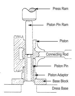
Section showing application of "Safe-T" Pin Removal Guide. (for piston pin .875-1.000 dia.)
