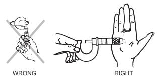
Note that the procedure requires two hands. If the micrometer is handled with only one hand, the ratchet stop cannot be reached, and reliability will suffer. It works out fine for any part that is large enough to support itself without moving around during measurement. It is awkward for small parts.
