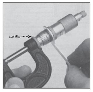
**CAUTION:** If the spindle is removed for cleaning, DO NOT touch the lock ring!
