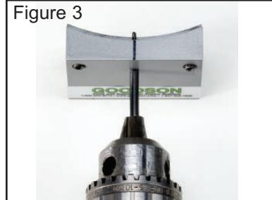
**Warning:** Drilling gas port deeper than ring groove can destroy the piston by drilling through piston valve reliefs or inside of piston.
