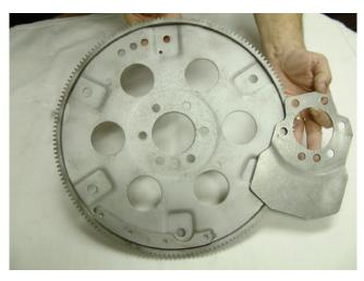
400 plate smooth 454 plate has addition of welded weight. Plates FBP-25, FBR-54 are not interchangeable
