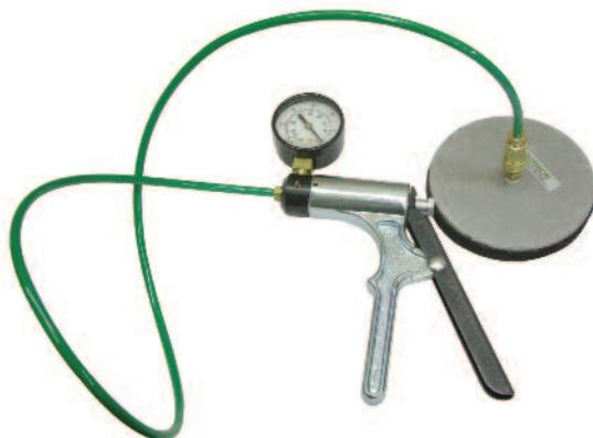
The **DVC-101-HD** Manual Vacuum Tester provides a quick, simple and accurate method for checking valve seating on most gasoline and diesel engines. A rubber 4  $\frac{3}{4}$ " adaptor is placed over the combustion chamber, vacuum is applied, and valve seating is checked by timing vacuum leak-down.
