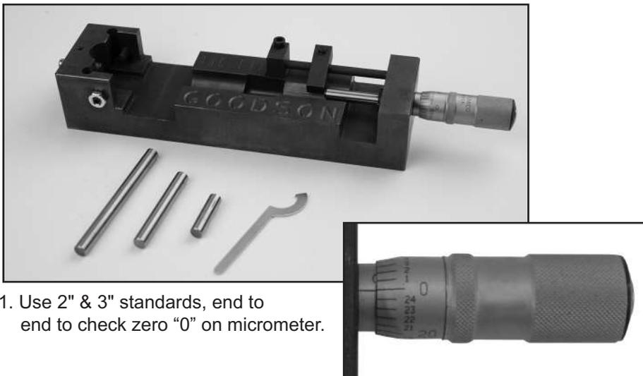
1. Use 2" & 3" standards, end to end to check zero "0" on micrometer.
