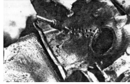
This photo shows a repair with the holes drilled and tapped. Here, where the metal in the casing is relatively thin, it is not usually necessary to use a tapered reamer before tapping the holes.
