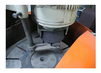
Always make sure your machine is level left to right and add a slight tilt forward for better draining of the grinding fluid or coolant.
