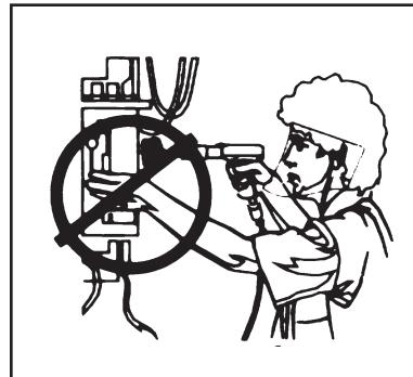
1. Remove rotor from car. Do not use die grinder or high speed drills.
