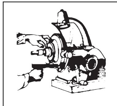
2. Mount rotor on brake lathe spindle. Rotate motor 125-210 RPM.
