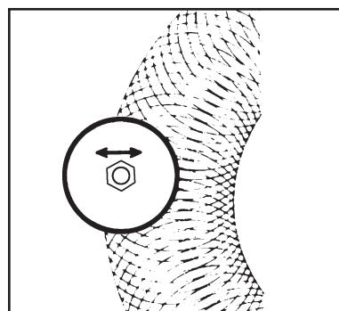
4. Stroke tool in towards center and out 8-10 times. For improved pattern, reverse tool rotation stroke 4 to 6 times.
