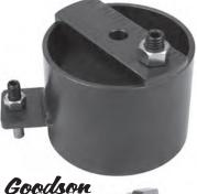
All steel construction features 2 indexing dowels to properly align the reluctor ring when installing it on the crankshaft. Designed to fit Generation III (LS1, LS6) and Generation IV (LS 2, LS3, LS7) engines. Aligns GM sensor rings (12559353, 12586768). US Patent No. 7,716,827.
