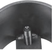
The internal indexing dowel pin is designed to fit into the dowel pin hole on the crankshaft. It is adjustable to fit different depths. The combination of dowel pins gives very precise alignment of the reluctor wheel and crankshaft.
