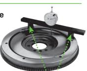
Magnetic feet adjust to flywheel diameter
