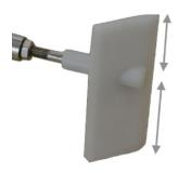
Place the stone holder in the drum and tighten the top lock nut, making sure the deflector blades don't touch the walls of the drum. Tighten the nuts of the deflector blades in place with spanner.
