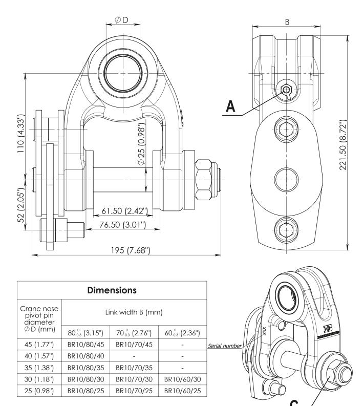
Max. Load - 5.5 ton (55 kN) Weight - 6.5±1 kg (14.5±2.2 lb)
