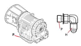
8 - Attach the hydraulic hose to the fittings (H). Check oil level and signs of oil leakage.
