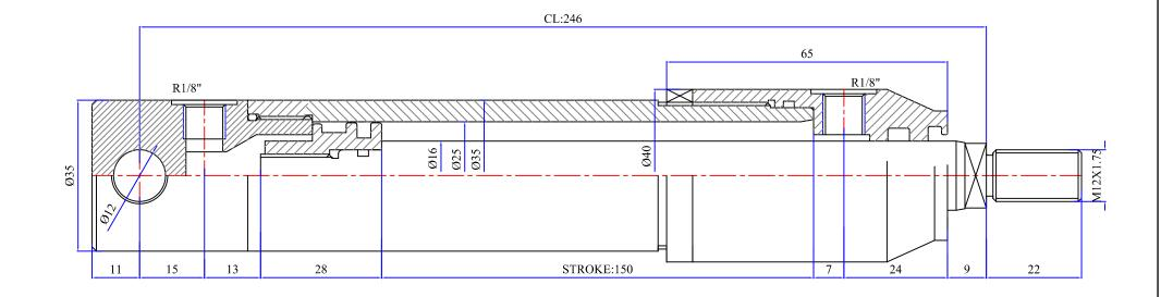
Part No. HP-71625-150 FINISHED ZINC PLATED MAX PRESSURE 210 BAR Test Pressure:
