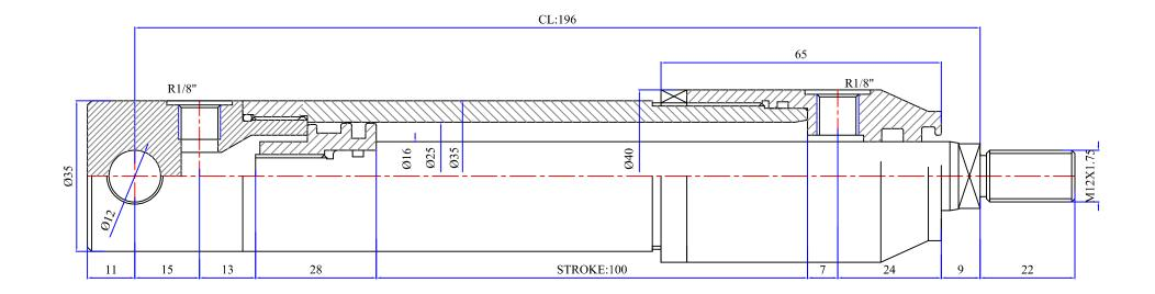
Part No. HP-71625-100 FINISHED ZINC PLATED MAX PRESSURE 210 BAR Test Pressure:
