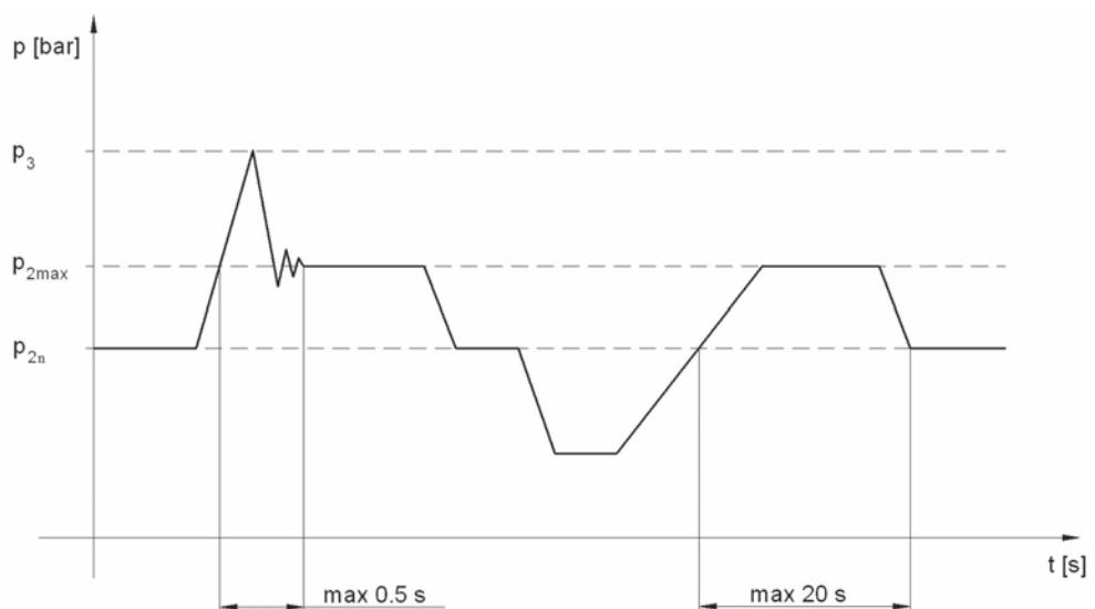
$p_{2n}$  max. contin. pressure Max. working pressure, at which the pump can be operated without time limitation.
