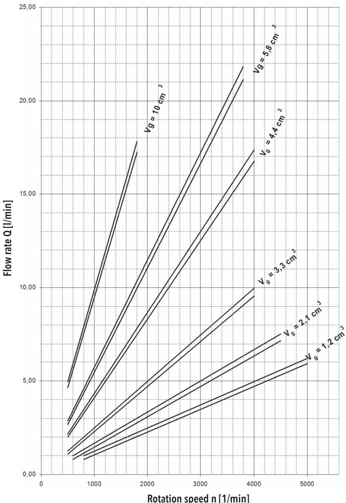
Above curves apply to ISO V<sub>g</sub> 46 oil at temperature  $t = 45^\circ\text{C}$ .
