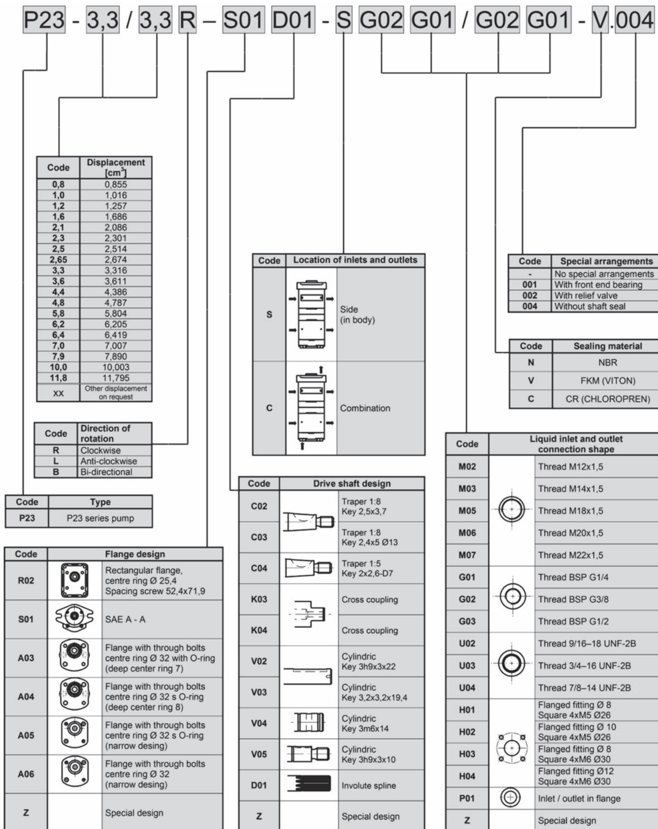
An example of designation for the P23 two-section clockwise pump with displacements of 4.4 and 3.3 cm<sup>3</sup>, rectangular flange, centre ring Δ 25.4, Trapper 1:8 with key 2.4x5 Δ 13, one common input and to outputs with metric threads, FKM sealing without special arrangements: **P23-4.4/3.3R-R02C03-SM05M05/NM05-V**
