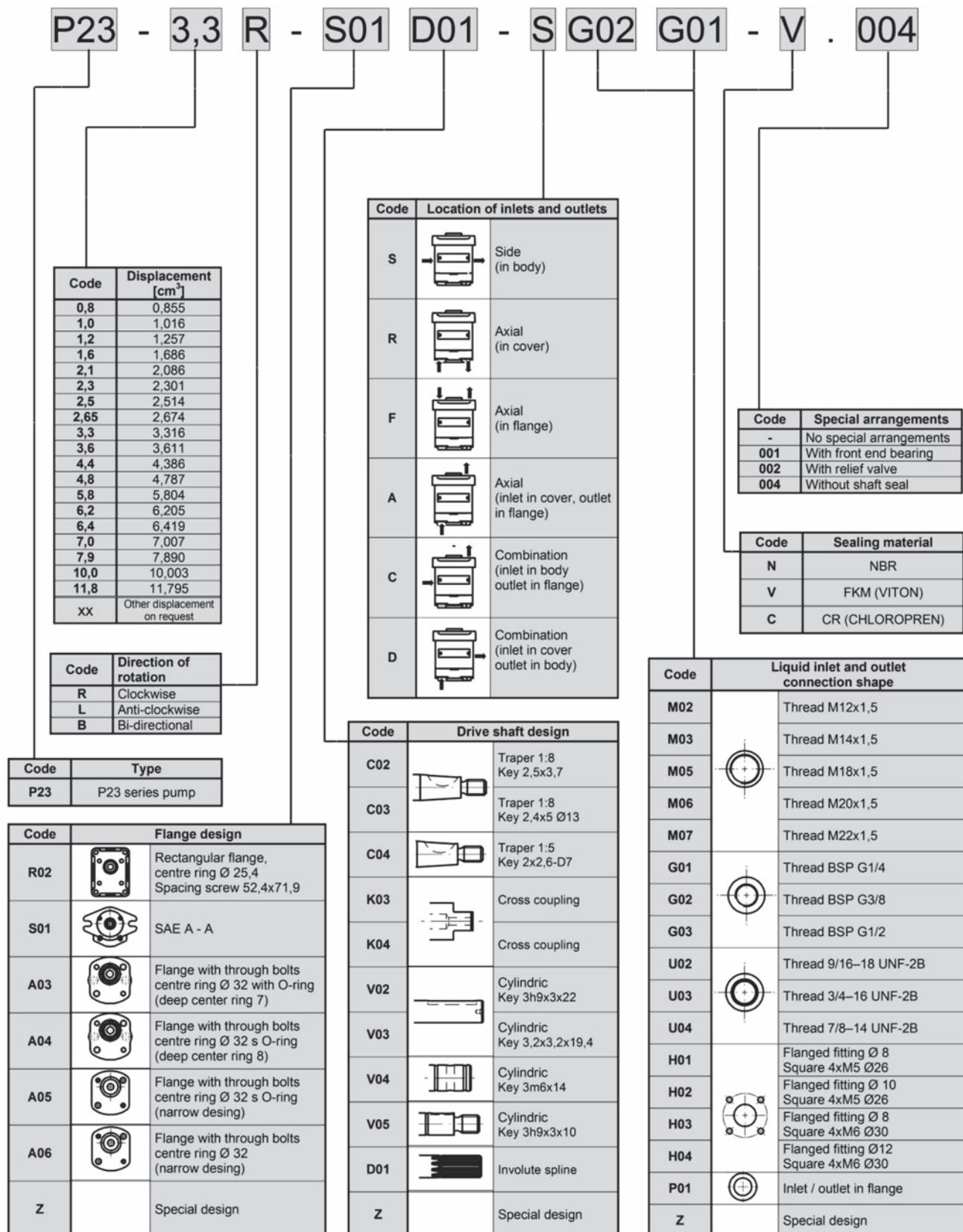
An example of designation for the P23 anti-clockwise pump with displacement of 4.4 cm<sup>3</sup>/rev, SAE A-A flange, trapper 1:8 with key 2.5x3.7, BSP side inlets and standard NBR seal without special arrangements: **P23-4.4I-S01C02-SG03G03-N**
