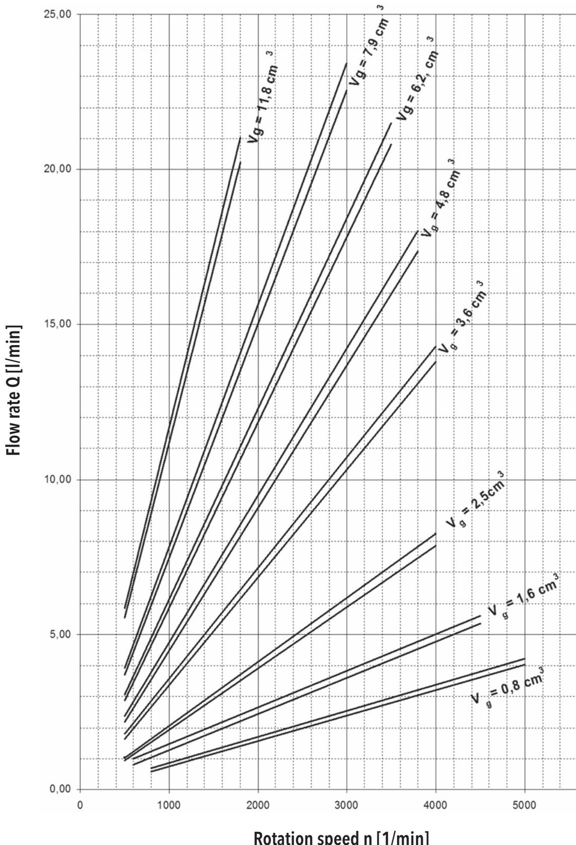
Above curves apply to ISO  $V_g$  46 oil at temperature  $t = 45^\circ\text{C}$ .
