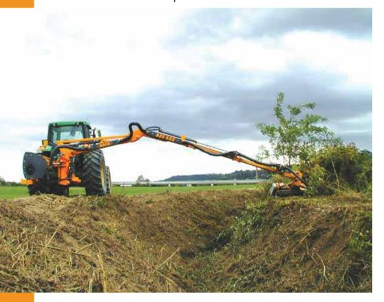
Hydraulic hedge mower of 8.9 m. range, for tractors HP 150/200 and weight 7000 kg, suitable for heavy drainage and road mowing, strong, compact, connected on the tractor in high position and fast on the motions.
