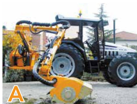
A: Machine with central advancement to the tractor, for a great visibility during work.
