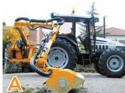
A: Machine with central advancement to the tractor, for a great visibility during work.
