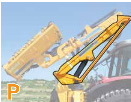
P: Mechanism that allows to work flush to the wheel with long extension machines, with a very-good speed and handling quickness.
