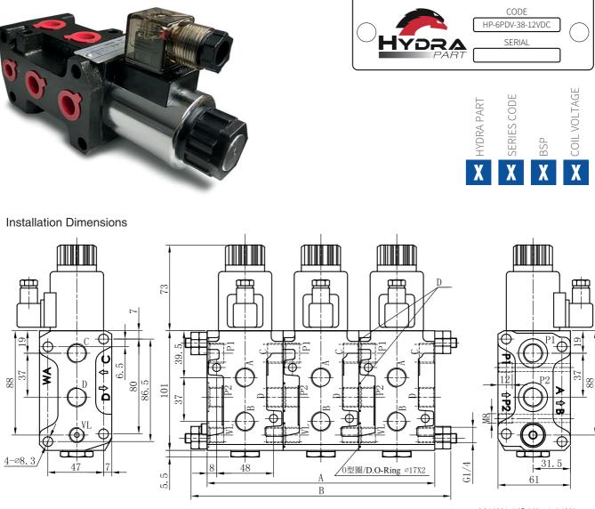
$\begin{array}{l} M18X1.5/G3/8 = \Phi\,21X2 \\ M22X1.5/G1/2 = \Phi\,23.5X2 \end{array}$
