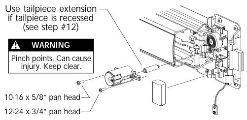
Install center case cover. **Use long** screws where shown for tamper resistance. Depress pushpad to install hinge side cover.
