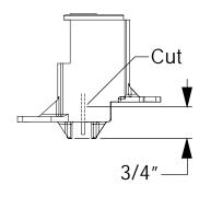
If tailpiece is recessed less than 3/4" cut for 3/4" recess and use extension in Step 14 Use Phillips screwdriver to rotate cross slots inside center case so marks align.
