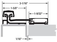
Model SL21 requires repositioning of existing overhead closer(s) to match the swing clear pivot point of the hinge. Failure to do so will prevent the door from opening more than 70 degrees. Attach hinge leaf cover before reinstalling closer(s).
