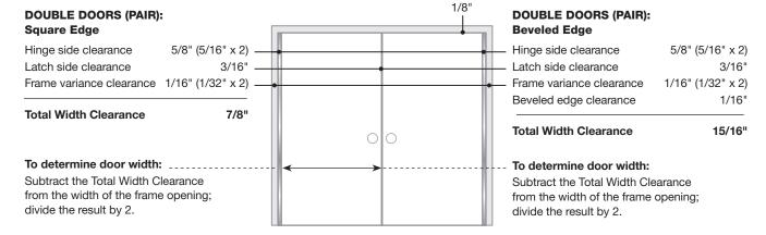
**NOTE:** For double-door entrances with a mullion <u>between</u> the pair of doors, calculate each door width using the Single Door clearances. For double-door entrances with a mullion <u>behind</u> the pair of doors, calculate each door width using the Double Doors clearances.
