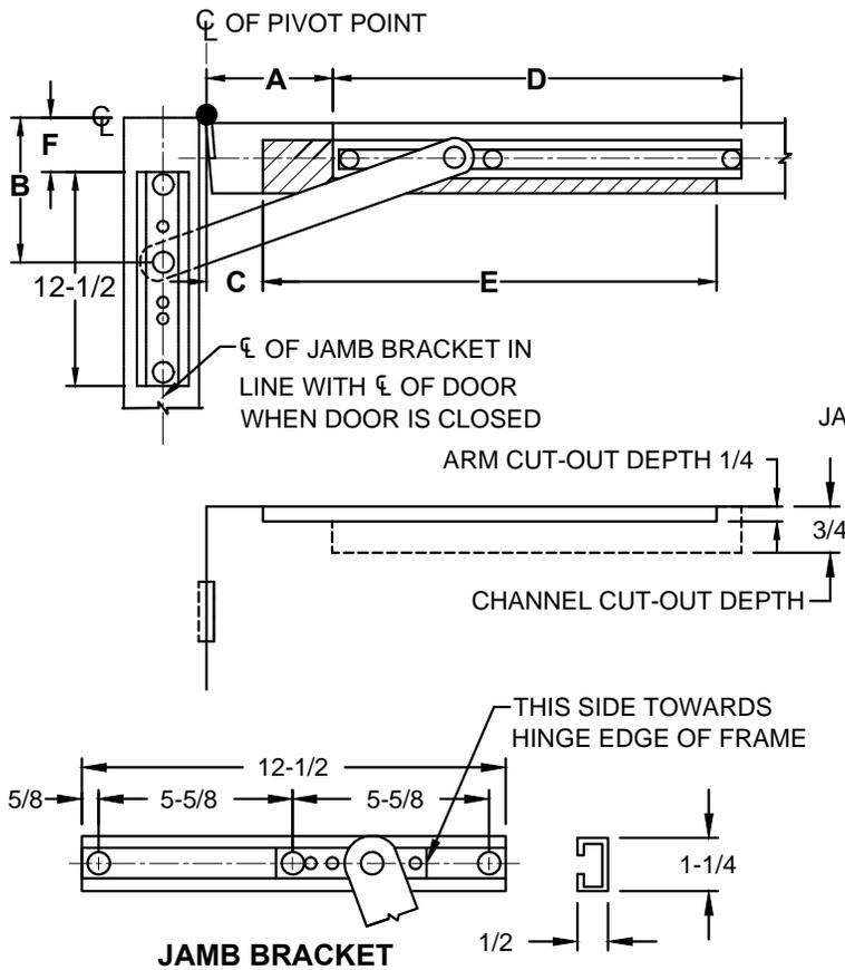
**A** =  $\epsilon$  OF PIVOT POINT TO START OF CHANNEL CUT-OUT
