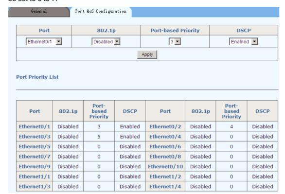
selected **Port**, if **802.1p** and **DSCP** is set to be enabled, the **Port-based Priority** can be set to 0 to 7.
