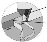
45 mm wide clear integrated adhesive tape on the underside of the membrane.
