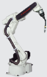
Robot 6 Axis 2.0 Meter Reach
