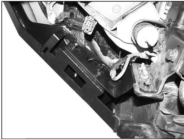
(Fig 15) Driver/left Wing installed
