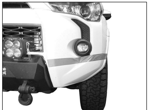
(Fig 4) Masking tape used to make a straight line from the front mark to the wheel opening. Follow bottom edge of masking tape
