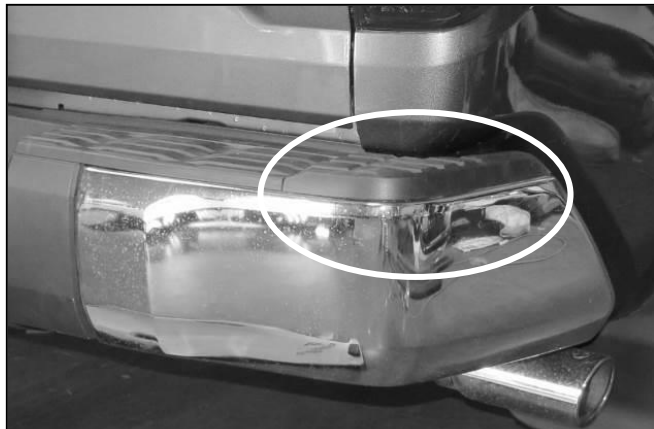
(Fig 3) Use a flat blade screwdriver to pry the plastic cover from the top of edges of the bumper
