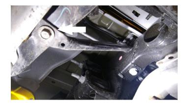
6. Remove the four 18mm nuts of the bumper brackets.
