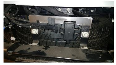
9. If the vehicle is equipped with A.D.A.S. (Advanced Driver Assist System) remove them from the factory bumper and mount to the two small holes located on the mounting bracket. You will need to drill the hole to ¼" and then mark and drill another hole in-line with the second hole of the bracket. Put the white plastic spacers between the mounting bracket and the ADAS bracket.
