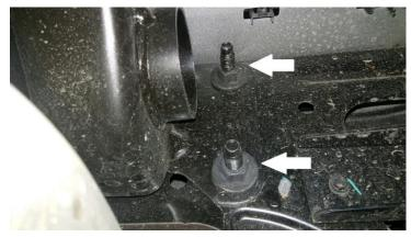
7. Remove the two 13mm bolts that are located behind the license plate and remove bumper.
