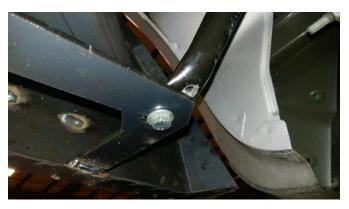
12. Center bumper from side to side and then tighten all bolts and nuts.
