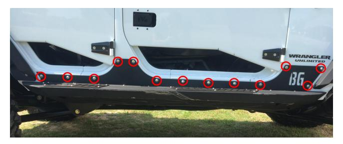
6. Next repleate STEP 2 by reinstalling step with body mounts. Next install body side trim using hardware from: J-HK-SS07 (26) 5/16"- $18 \times 3/4$ " Long, Stainless Steel SBHCS
