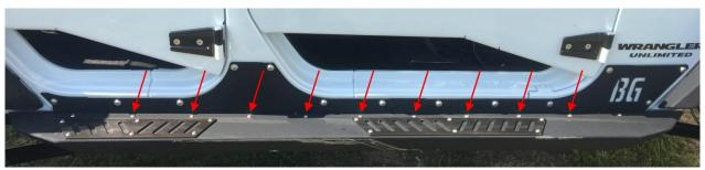
5. Install the rest of the 1/4-20 x 5/8 Long bolts to secure body trim to step.
