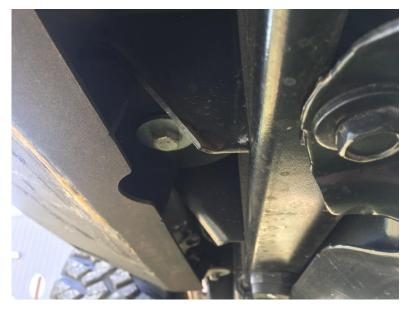
2. Next remove three body mounts and then install step onto jeep using body mounts.
