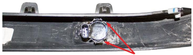
Release the parking sensor by spreading these two tabs
