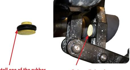
Install one of the rubber grommets onto it
