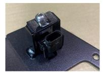
Note: Do not over tighten sensors. If sensors are not working properly, use CRC Dielectric grease PN#05113 on all sensors and main harness plug.
