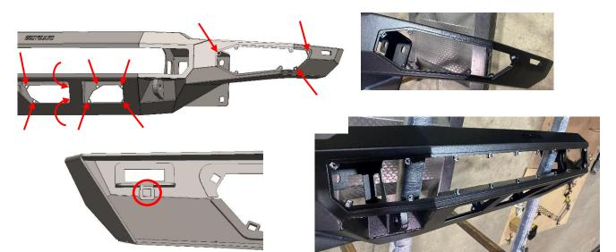
2. Carefully place the bumper up to the frame and fasten using 7/16"-14 hardware. Adjust fitment vertically and horizontally, then tighten all hardware.
