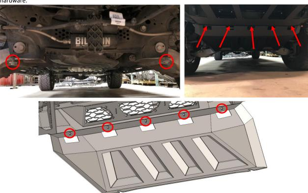
6. If applicable, install light bar with the light bar brackets, or light pods with the spacers in the positions indicated.
